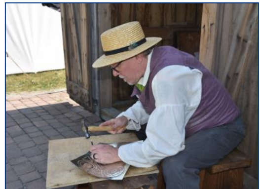
Brian Kilmer, Master Tinsmith, working on the punched tin panels (here and left)
