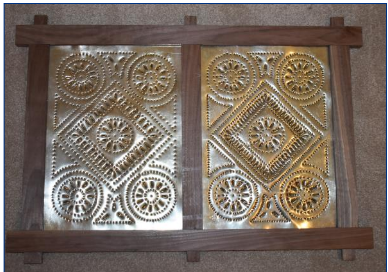
Dry fit complete. Time to take it apart and drill peg holes.
