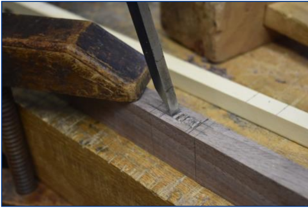
Making the first pass of cutting a mortis, a rectangular socket in the stiles that accepts a tenon cut on the ends of the rails.
